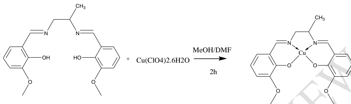
Scheme 4. Reaction scheme for the synthesis of the copper (II) complex
