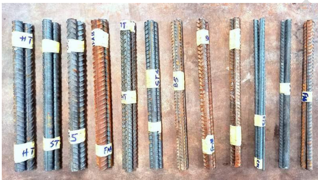
Fig. 3: Samples of the Reinforcements Prepared for the Mechanical Properties Test
