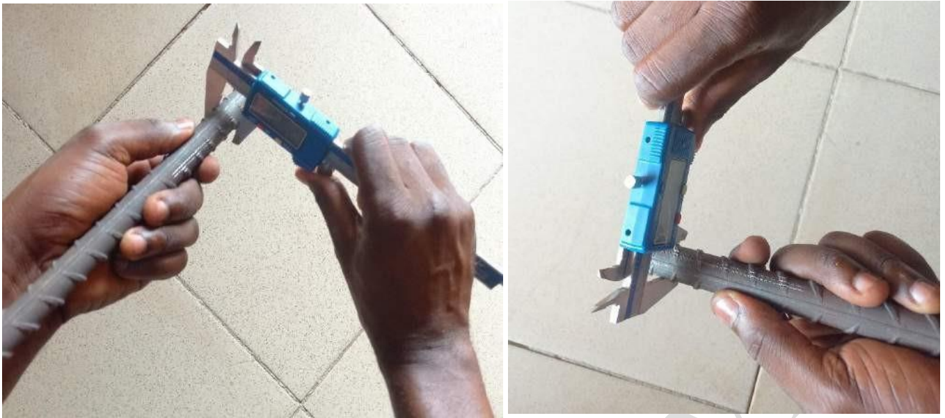
Fig. 2: Measuring the Diameter of a Reinforcing Steel Bar with a Vernier Caliper
