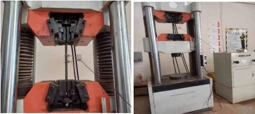
Fig. 4 Testing Steel Bars to find the Mechanical Properties of Reinforcement with an Avery Denison Universal Testing Machine-
