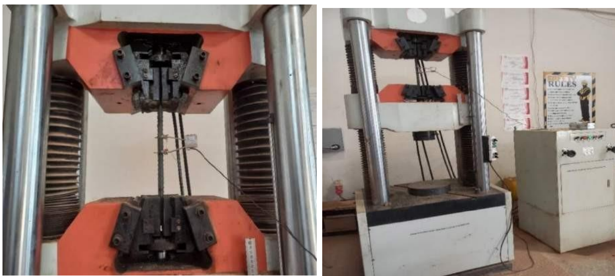
Fig. 4 Testing the Mechanical Properties of Reinforcement with an Avery Denison Universal Testing Machine.
