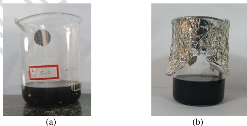
Figure 2. Samples in solvent (a) o-Xylene & (b) Toluene after treating for 1 hour at 80°C
