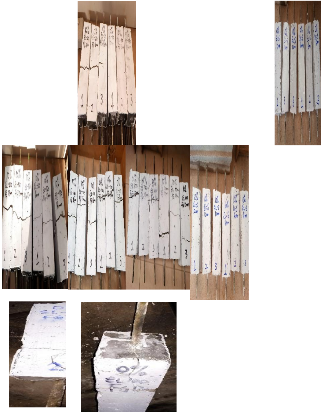
Figure 10: Tested double pull-out prism specimens with GFRP rebars.
