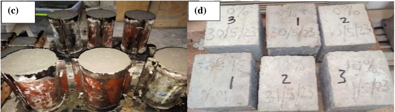
Fig. 3: Specimens: (a) Prism specimens, (b) Hardened prism specimen, (c) cylindrical specimens, (d) cube specimens
