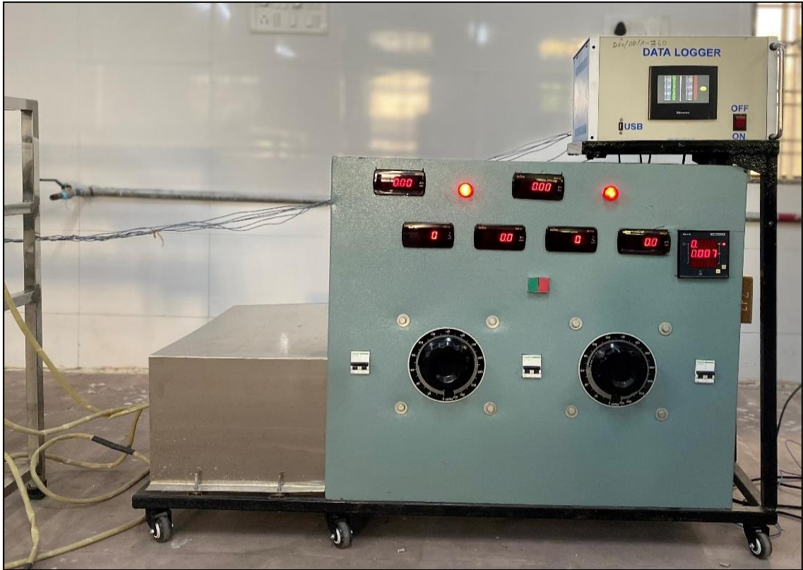
Figure 5: Control panel for continuous ohmic heater
