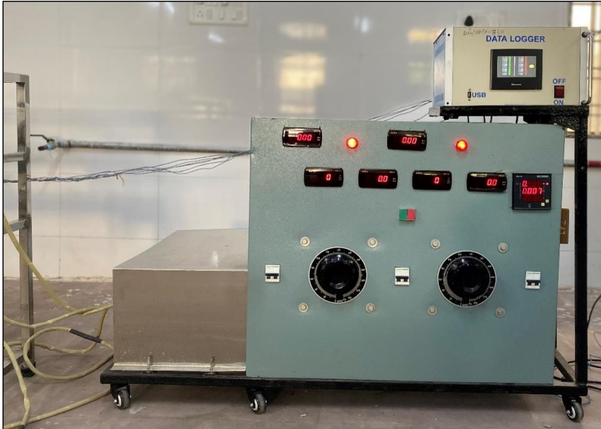
Fig 5: Control panel for continuous ohmic heater
