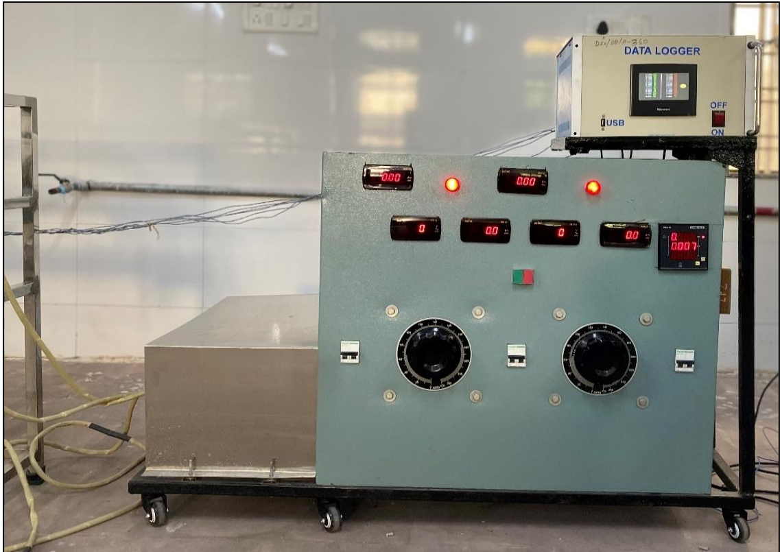
Fig 5: Control panel for continuous ohmic heater
