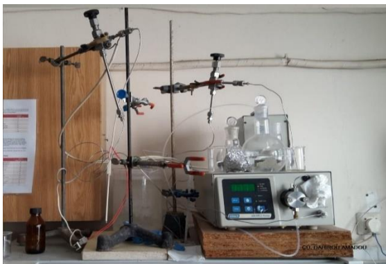
Figure 5: Superheated water extraction device and Schematic diagram
