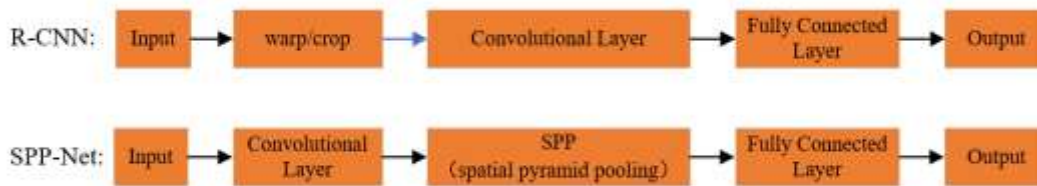
Figure 4: Comparison of the process between SPP-Net and R-CNN algorithms.
