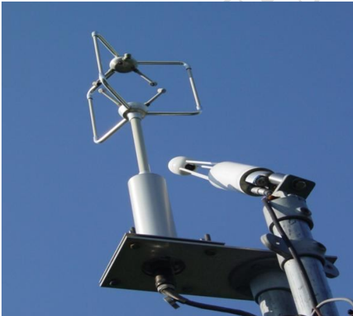
146 147 Figure 6: Eddy Covariance Towers for Gas Exchange Monitoring
