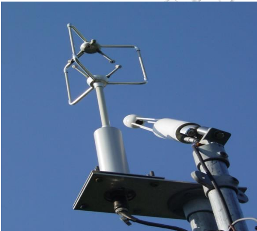
Figure 6: Eddy Covariance Towers for Gas Exchange Monitoring
