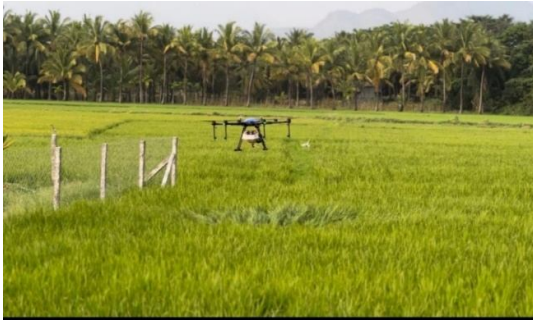
Figure 1: - Air spraying of pesticide with the help of drone
