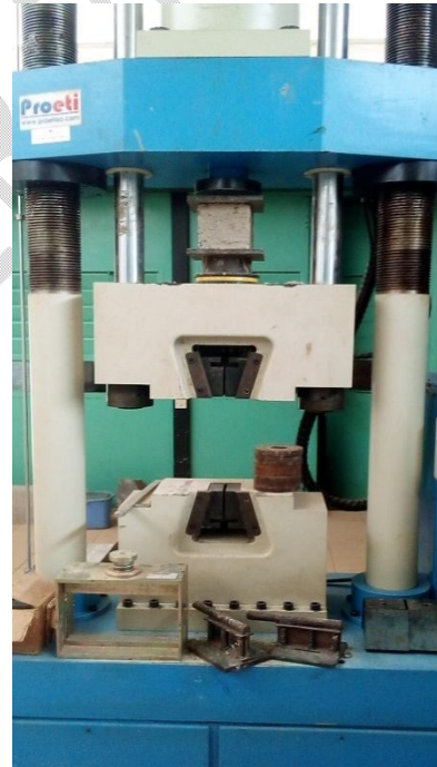
(a) Concrete cube under test
