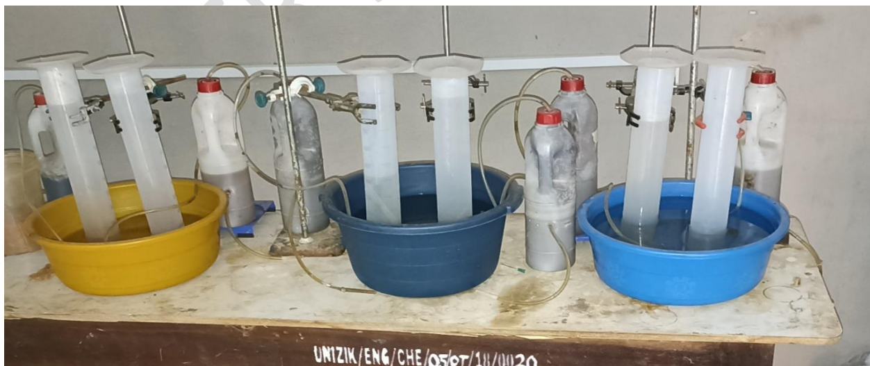
Fig. 1: The laboratory setup of anaerobic digestion
