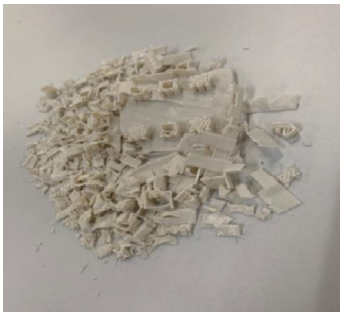
Figure 3. Manually removed Infills
