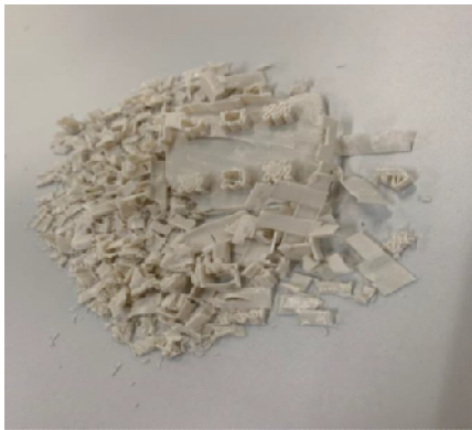
Figure 3. Manually removed Infills
