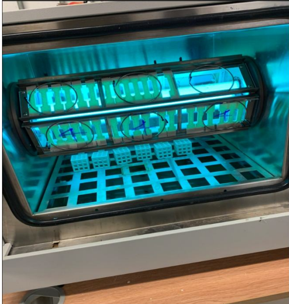
Figure 4. BGD 852 Bench UV Accelerated Cabinet with first sets of cubes under UV Light
