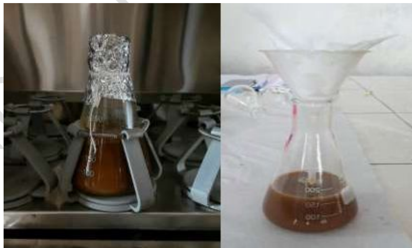
Figure 3: Broth kept in overnight BOD incubator shaker and filtered using muslin cloth.
