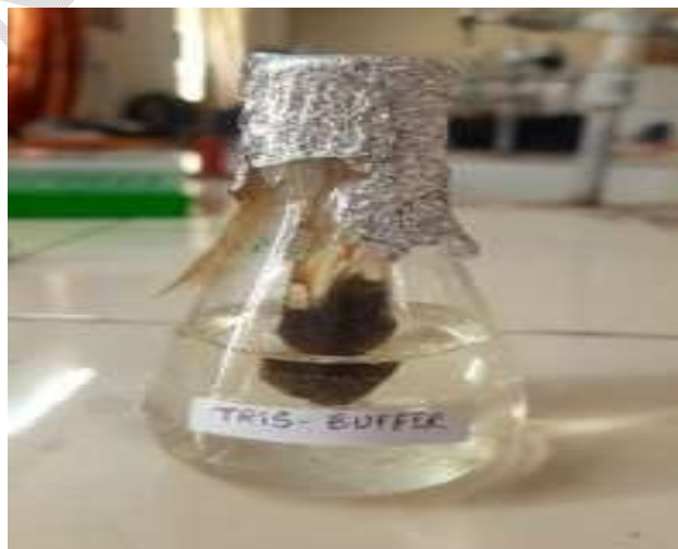
Figure 9: Conical flask containing Tris buffer and dialysis bag with enzyme inside.
