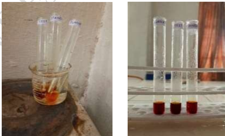
Figure 7: Blank, Test and Standard test tubes placed in boiling water bath and after that.
