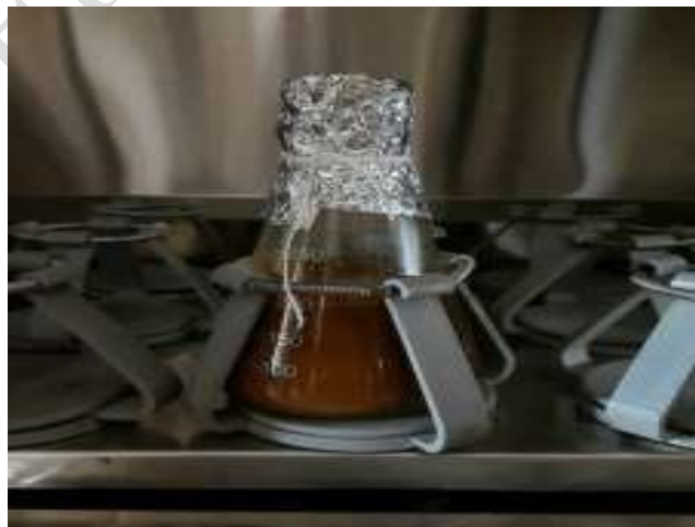
Figure22: Broth kept for fermentation in BOD incubator shaker
