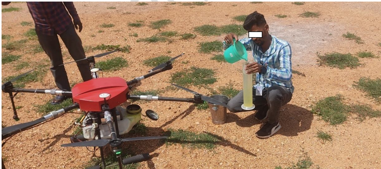
Figure 5. Determination of application rate of drone mounted sprayer various forward speed and height of spray under laboratory conditions
