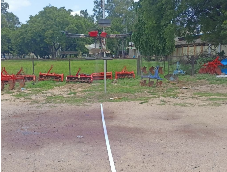
Figure4. Measurement of swath width of UAV at different height
