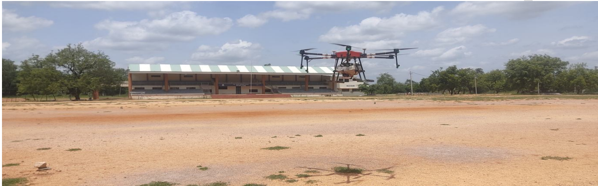
Figure 3. Determination of application rate of drone mounted sprayer various forward speed and height of spray under laboratory conditions
