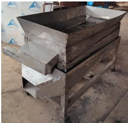
Fig. 4: Fabricated Double-Layered Grain Sieving Machine
