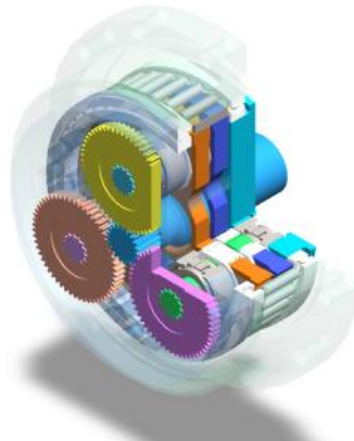
Fig. 2. Cutaway view of 2K-V reducer
