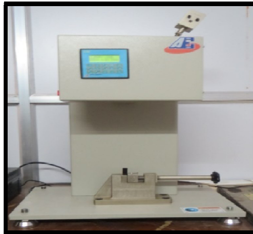
Fig. 6. Impact testing machine
