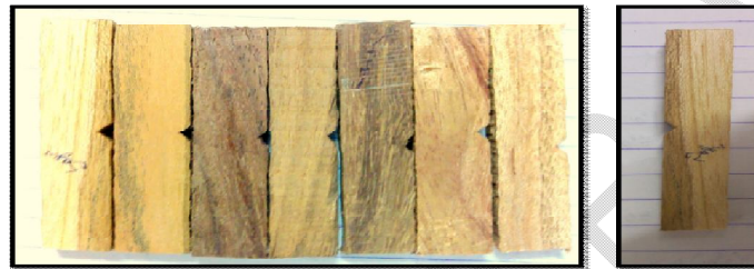
Figure 5: Prepared specimens for Impact test
