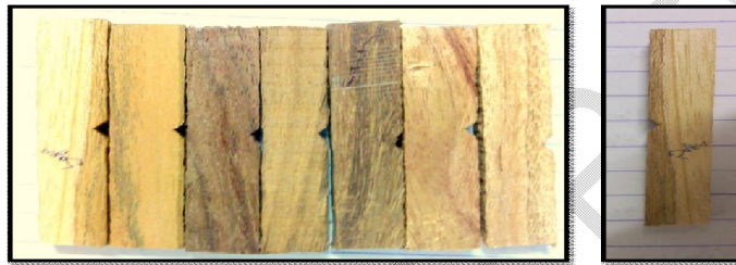
Figure 5: Prepared specimens for Impact test
