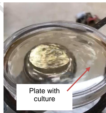
Fig 1. a) Experimental design of groups (Canva). b) Ultrasound equipment (model Sonomed V, CARCI, frequencies 1 MHz and 3 MHz), with transducer and plate without culture medium with water-based coupling gel. c) Application of ultrasound in liquid culture medium (Sabouraud Dextrose broth), Source: Personal archive.
