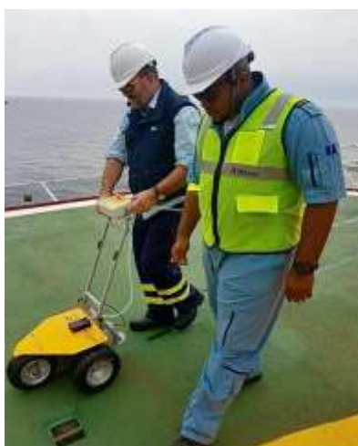
Fig. 3. Helideck inspectors operating the Findley Irvine equipment
