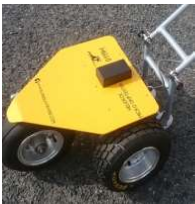
Figure 43: Findley Irvine Micro GripTester
