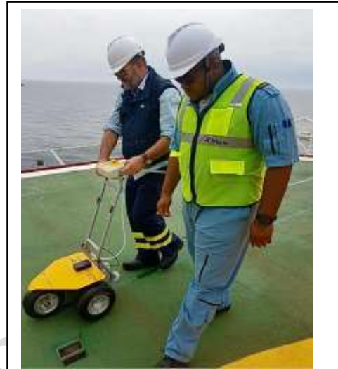
Figure 3: Helideck inspectors operating the Findley Irvine equipment.
