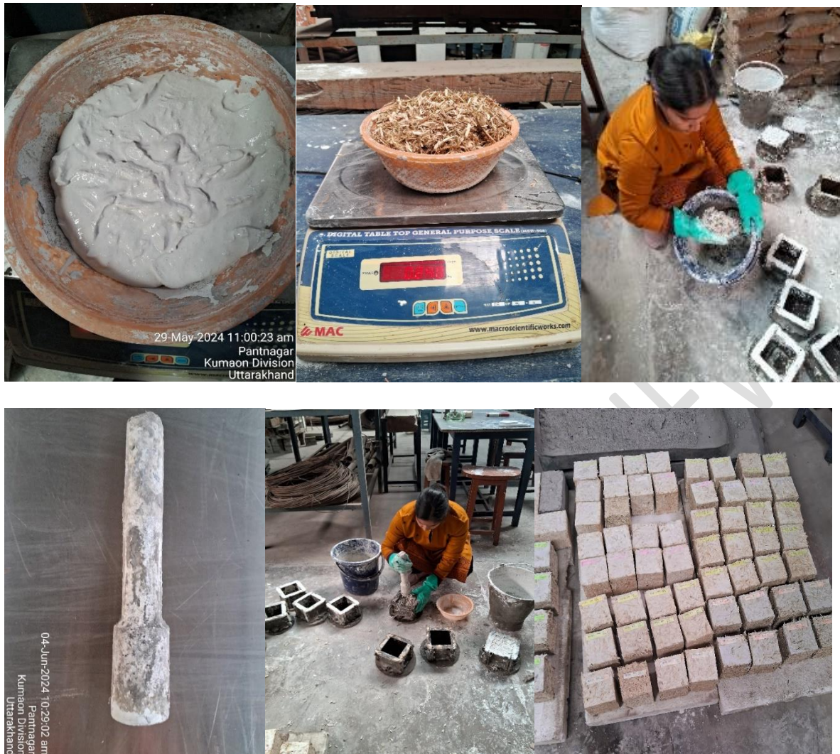
Figure 4. Pictorial presentation of production of concrete (a) Slaked lime paste (b) Weight batching of shiv (c) Mixing of lime and shiv (d) Iron rod used for compaction (e) Compaction of concrete into the cube mould (f) Final view of hempcrete cubes.
