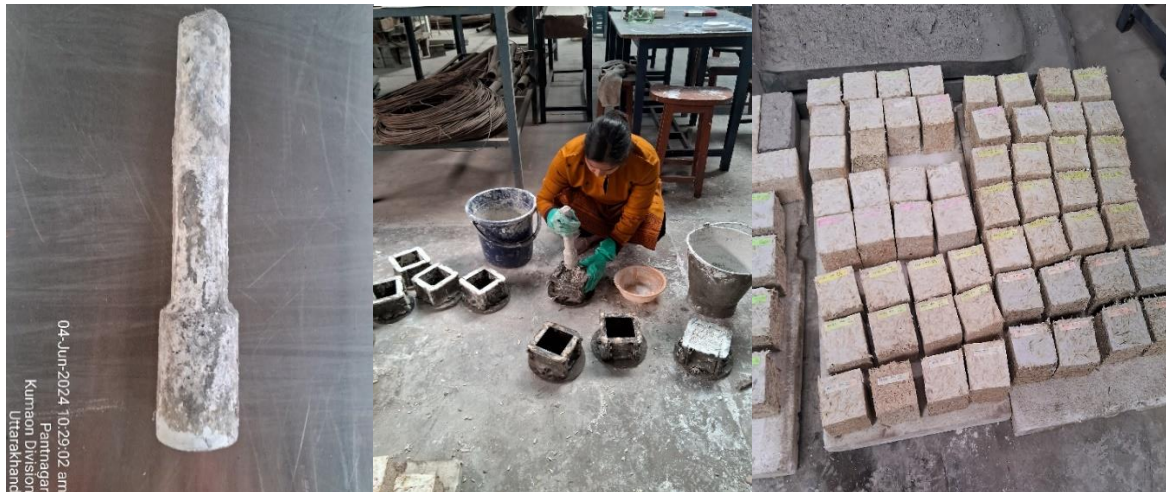
Figure 4. Pictorial presentation of production of concrete (a). Slaked lime paste (b) Weight batching of hemp shiv (c) Mixing of lime and shiv (d) Iron rod used for compaction (e) Compaction of concrete into the cube mould (f) Final view of hempcrete cubes.
