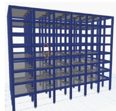
Fig. 3 Details of the Model with Static column removal for Flat Slab with Drop Panel Building
