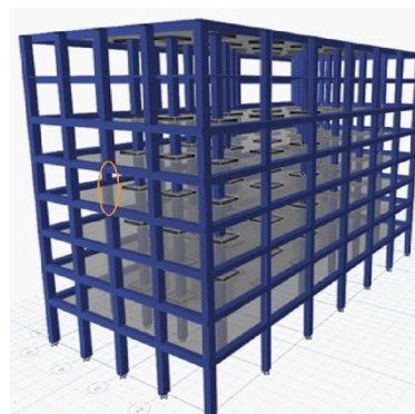
Fig. 3 Details of the Model with Static column removal for Flat Slab with Drop Panel Building
