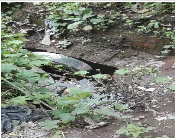
Fig .3 The leachate is distributed around the landfill in the lower part.
