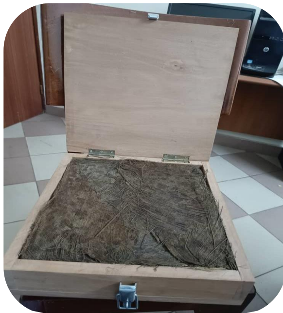
Fig. 7. Insulating panel sample with storage box
