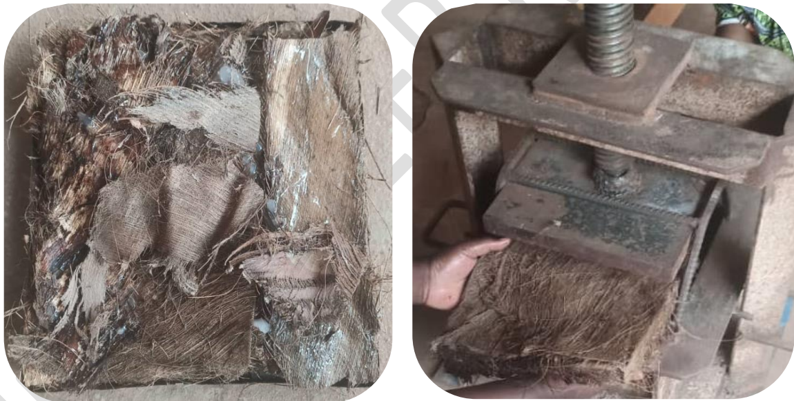
Fig. 6. Main stages in the production of insulation panels
