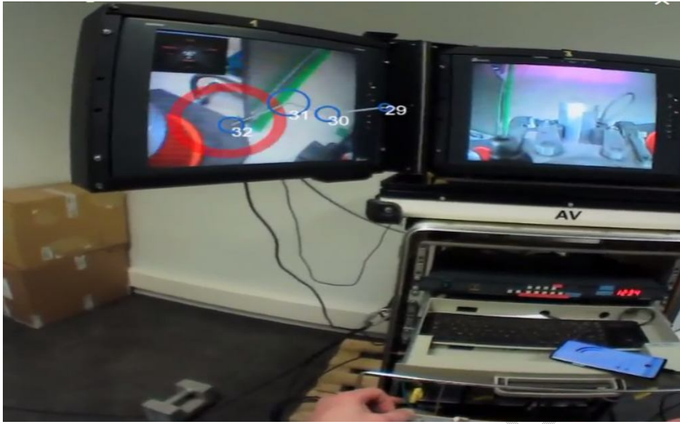
Fig. 6. Screenshot of the eye-tracking video recording and localization of the gaze (red circle) and fixation points (blue circles)
