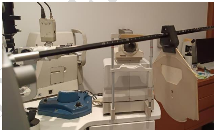
Figure 3: The distance of 35 cm at which the near-visual acuity chart was placed as the target.
