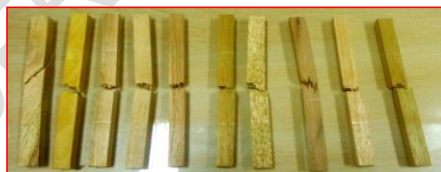
147 Figure 4: Test specimen of timber after testing
