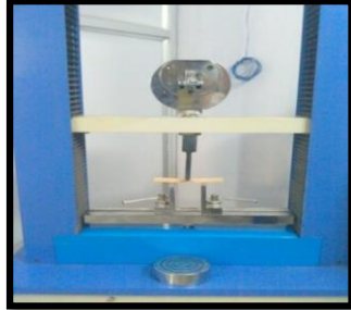
Figure 3: Test setup for Flexural strength
