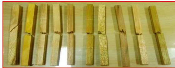
Figure 4: Test specimen of timber after testing
