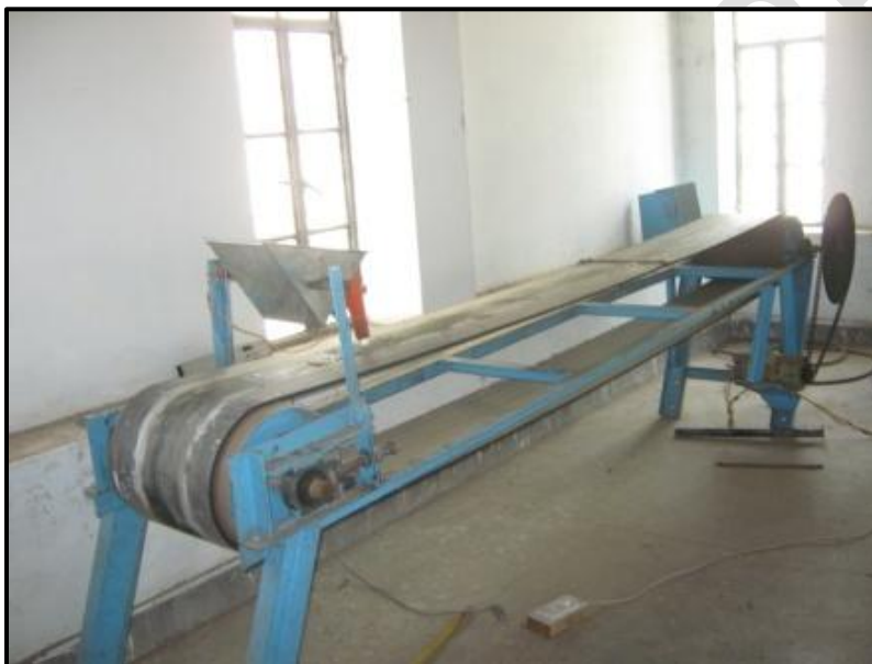
Fig. 2: Grease belt setup with opto- electronic sensor mounted on metering unit for laboratory testing.
