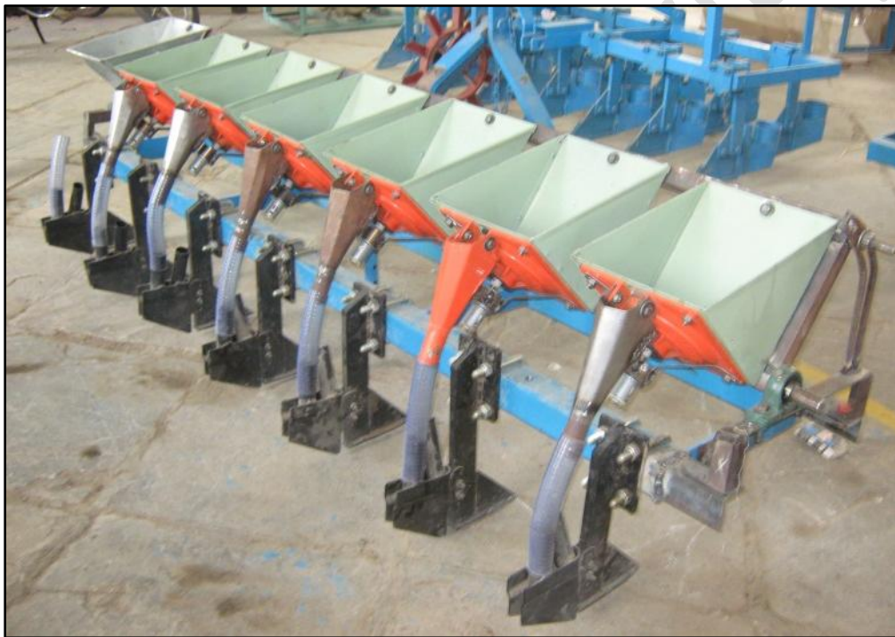
Fig. 3: Complete prototype unit of the seven rows electronic planter
