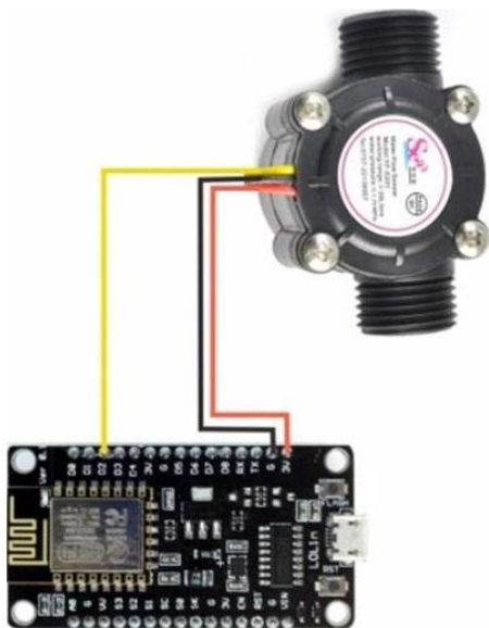
Figure 2: Flow Sensor Connected to Microcontroller
