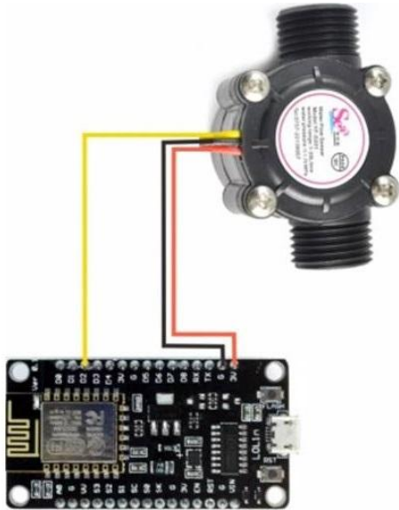
Figure 2: Flow Sensor Connected to Microcontroller
