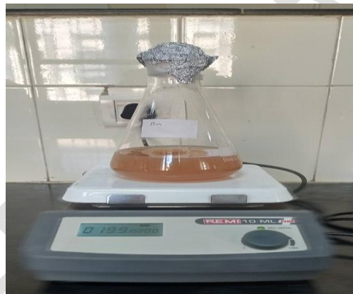
Figure 3 Interval shaking on magnetic stirrer
