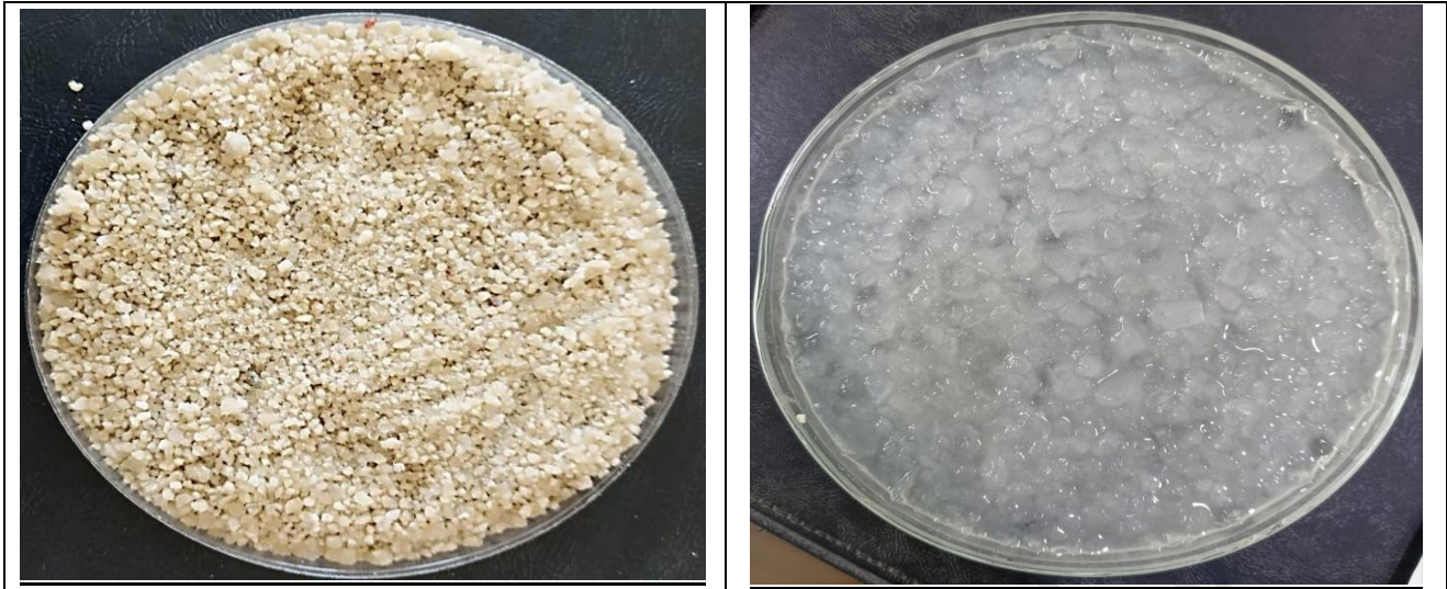
Fig(1): Hydrogel polymer before and after water absorption.
