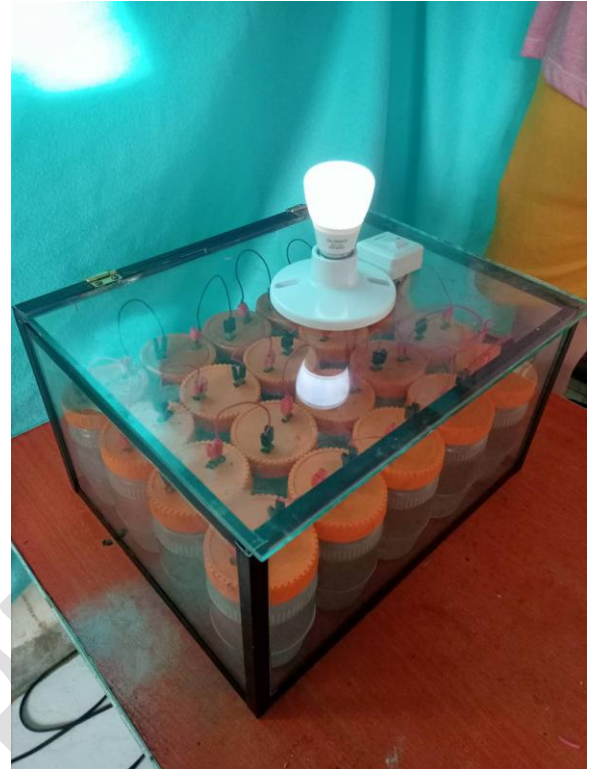
Figure 21 – Actual setup of a functional electrolytic cell with load
