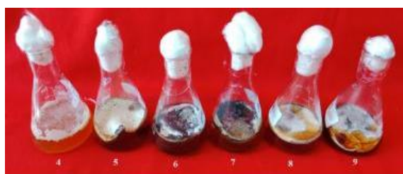
Fig. 7: Effect of Hydrogen ion concentration (pH) on the growth of P. palmarum on potato dextrose broth
