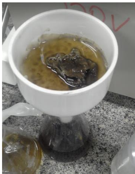
Fig. 3. Vacuum filtration of the fungus in a homemade medium.
