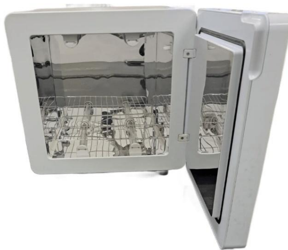
Fig. 3: UV-C light chamber with reflectors
